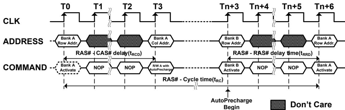
**Figure 3. BankActivate Command Cycle (Burst Length = n)**
