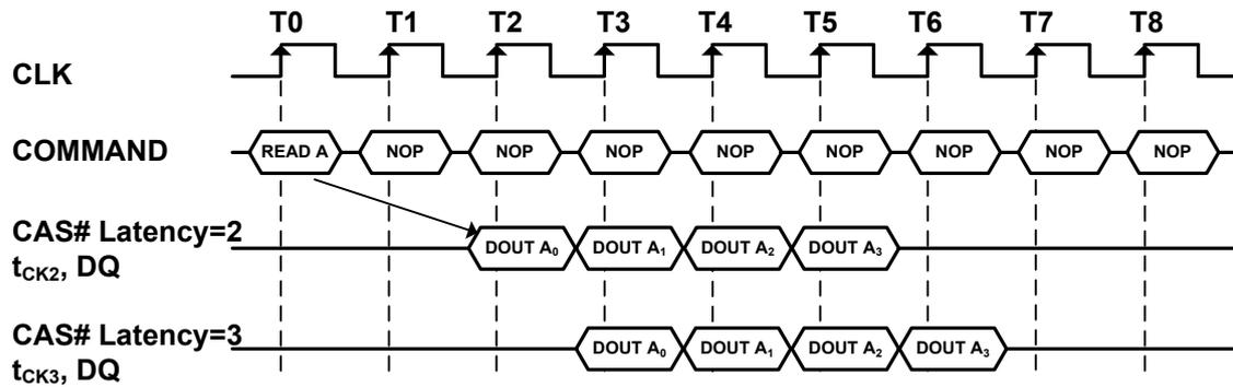
**Figure 4. Burst Read Operation (Burst Length = 4, CAS# Latency = 2, 3)**
