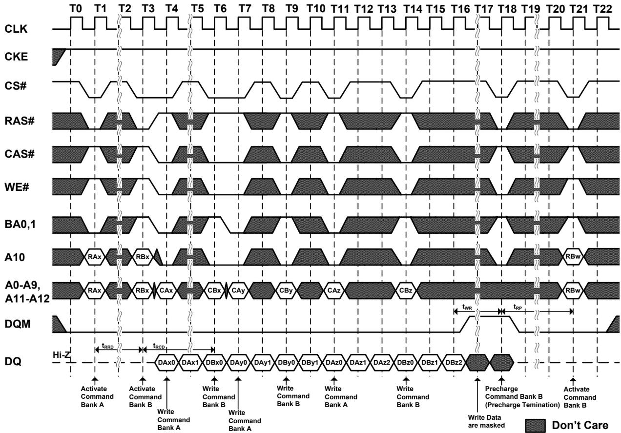
**Figure 42. Precharge Termination of a Burst**
