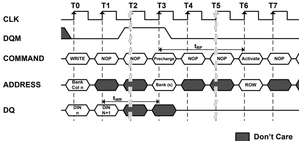
**Note:** The DQM can remain low in this example if the length of the write burst is 1 or 2.
