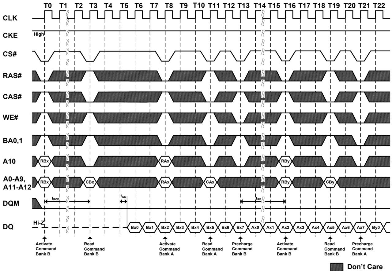
**Figure 30. Random Row Write (Interleaving Banks)**
