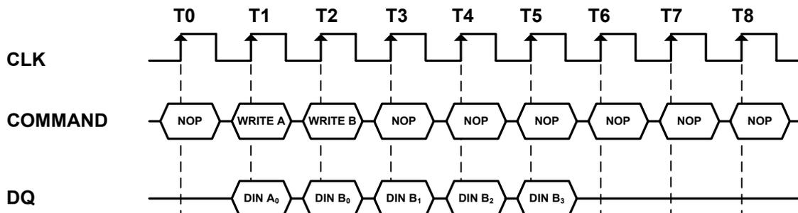
**Figure 11. Write Interrupted by a Write (Burst Length = 4)**
