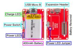
Battery Block Functional Diagram TOP
