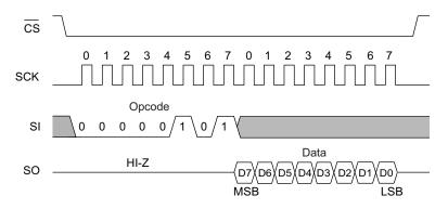
Figure 9. WRSR Bus Configuration (WREN not shown)
