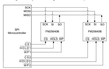
Figure 2. System Configuration with SPI port
