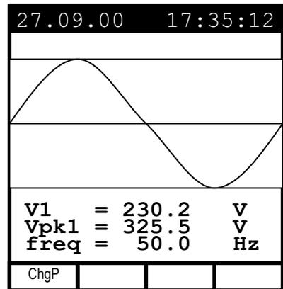
**Example of screen in "4-wire" three-phase system**
