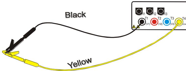
Connection of instrument terminals during calibration procedure.
