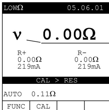
ATTENTION:  $R_{CALIBRATION} > R_{MEASURED}$
