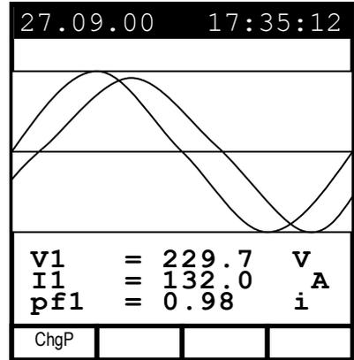
**Example of screen in "4-wire" three-phase mode**
