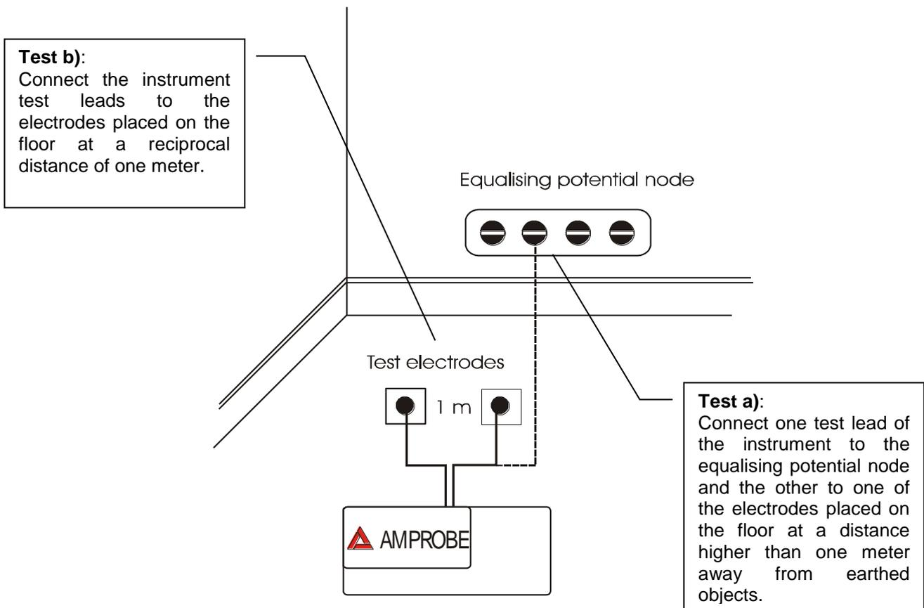
**Measurements of floor insulation resistance in medical rooms**
