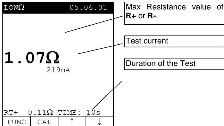
**Note:** We recommend the use of alligator clips and to assure the alligator clips make good contact with the conductor under test. Indeed, in this test the instrument gives as a final result the maximum measured value of R+ or R- and using test leads instead of alligator clips could give you faulty results due to faulty contact between the test leads and conductor under test
