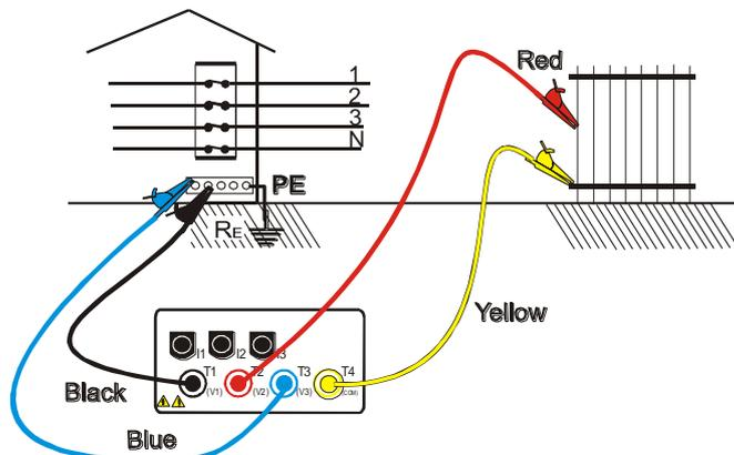
Connection for measuring the resistance between an extraneous conductive part and the earth system
