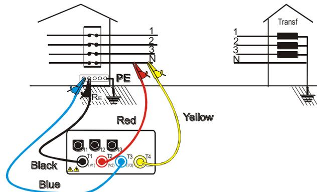
Connection for 2 point Earth Resistance measurement
