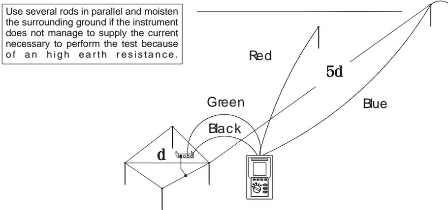
**Ground resistance measurement for small Ground plant**
