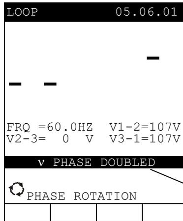
Two phases are connected together.
