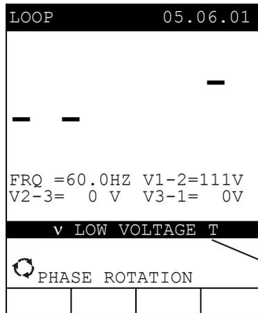
Phase "T2 Voltage is lower than 100V"
