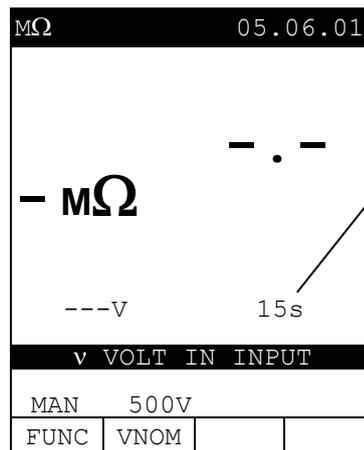
ATTENTION: the test can't be executed. Check that the circuit is not energized.
