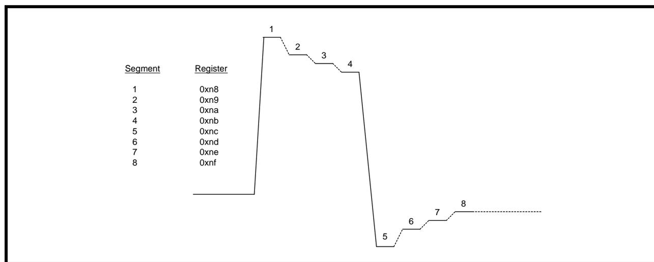
**NOTE:** By default, the arbitrary segments are programmed to 0x00h. The transmitter outputs will result in an all zero pattern to the line. For E1 arbitrary mode, see global register 0xC0h.
