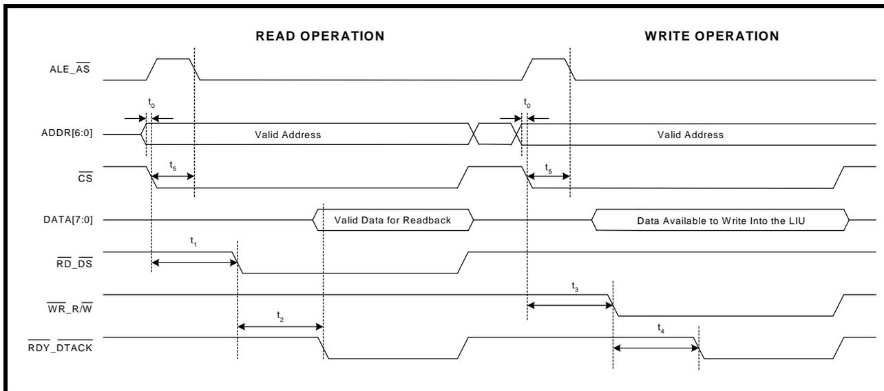
TABLE 56: ASYNCHRONOUS MODE 1 - INTEL 8051 AND 80188 INTERFACE TIMING
