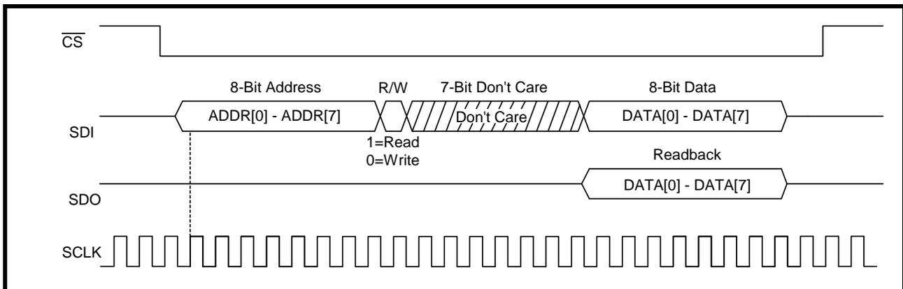
**NOTE:** For applications without a free running SCLK, a minimum of 1 SCLK pulse must be applied when  $\overline{CS}$  is “High”, before pulling  $\overline{CS}$  “Low”.
