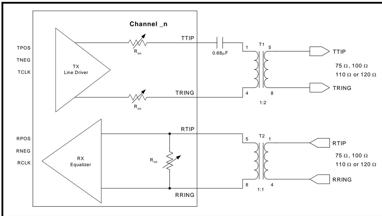
If the internal termination mode (RXTSEL = “1”) is selected, the effective impedance for E1, T1 or J1 can be achieved either with an internal resistor or a combination of internal and external resistors as shown in [Table 7](#).
