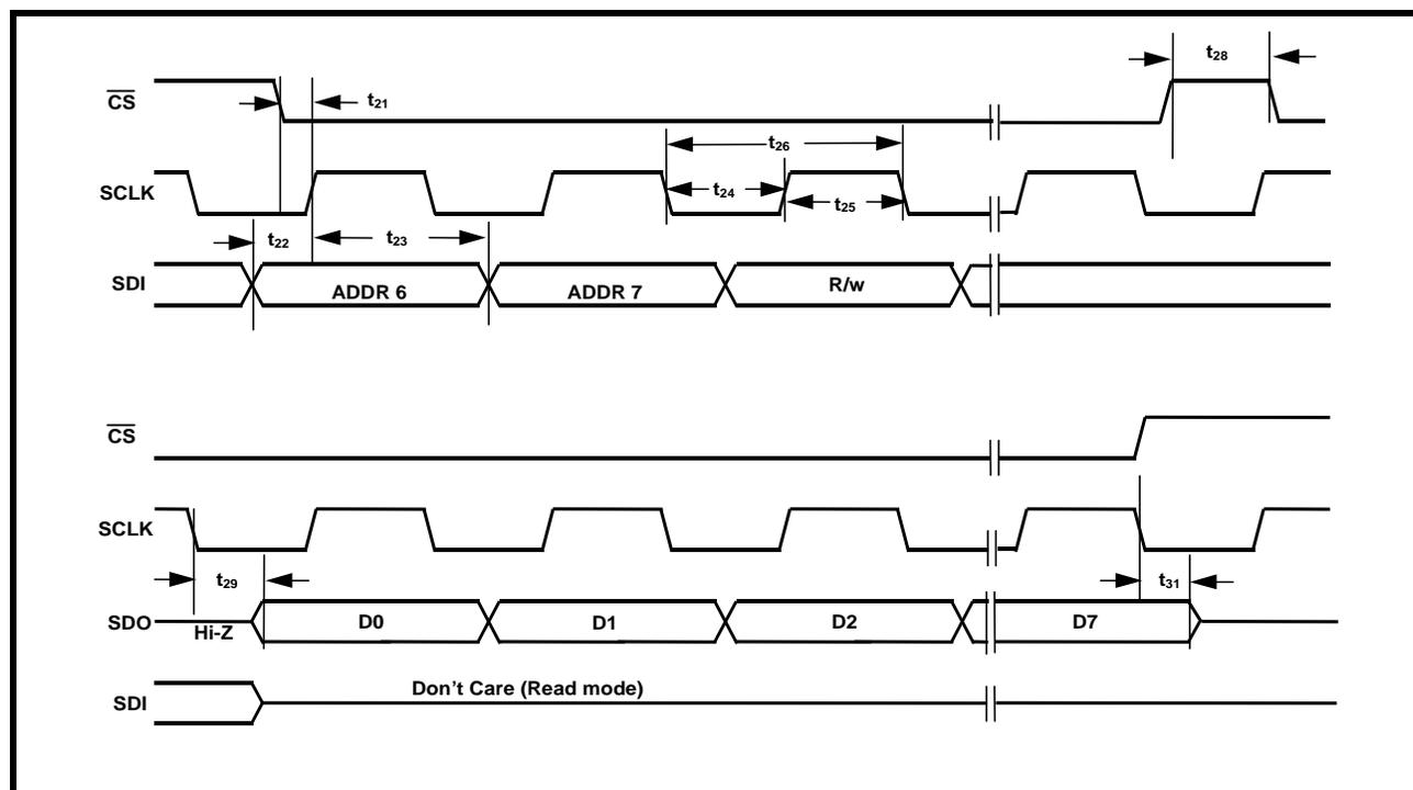
TABLE 14: MICROPROCESSOR SERIAL INTERFACE TIMINGS (  $T_A = 25^{\circ}\text{C}$ ,  $V_{DD} = 3.3\text{V} \pm 5\%$  AND LOAD = 10PF)
