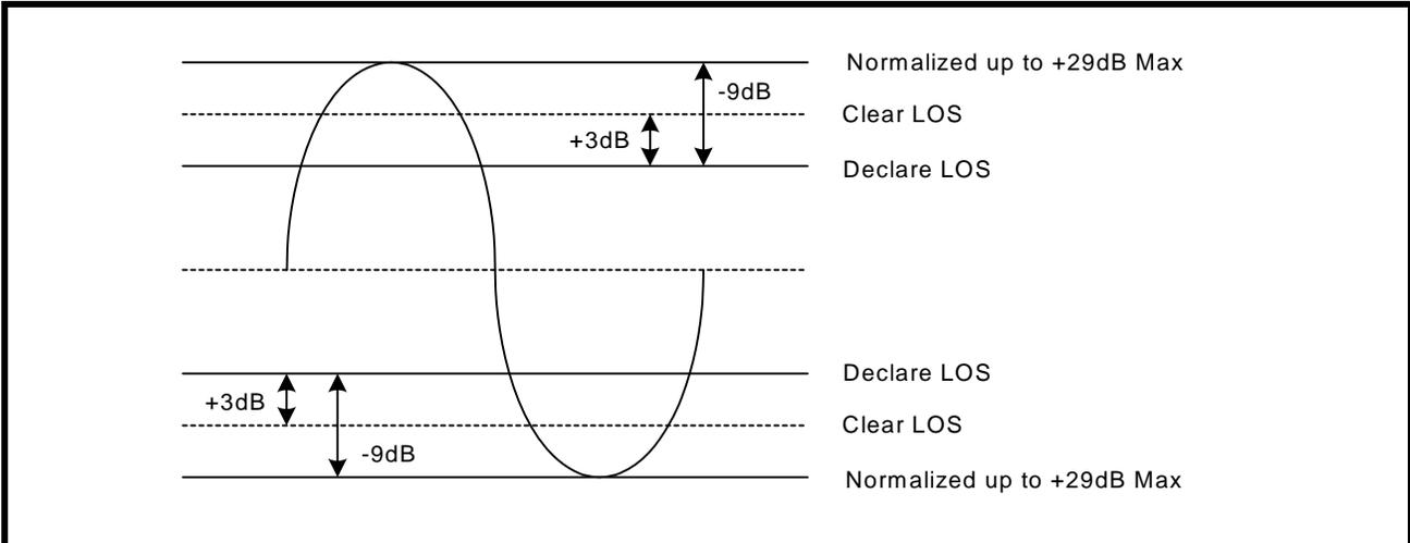
**Setting the Receiver Inputs to -36dB T1/E1 Long Haul Mode**
