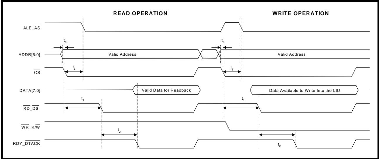
**TABLE 57: ASYNCHRONOUS - MOTOROLA 68K - INTERFACE TIMING SPECIFICATION**
