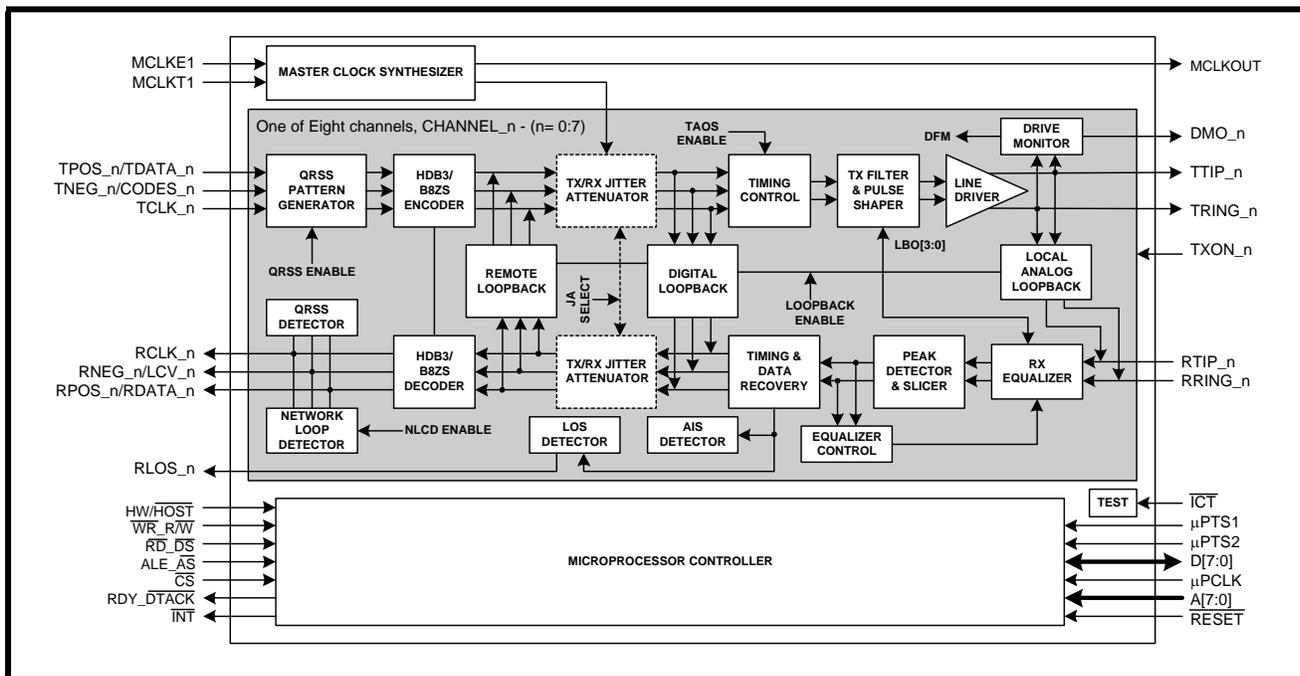
FIGURE 2. BLOCK DIAGRAM OF THE XRT83VL38 T1/E1/J1 LIU (HARDWARE MODE)
