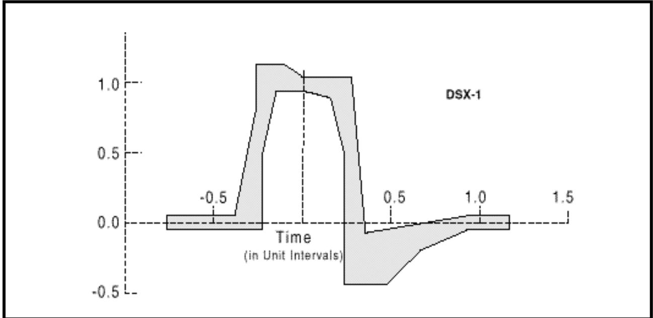
TABLE 54: DSX1 INTERFACE ISOLATED PULSE MASK AND CORNER POINTS
