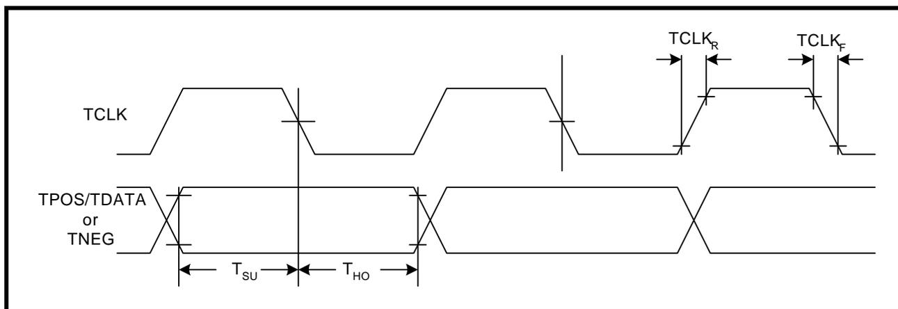
FIGURE 36. RECEIVE CLOCK AND OUTPUT DATA TIMING
