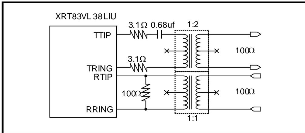
**FIGURE 15. SIMPLIFIED DIAGRAM FOR E1 IN EXTERNAL RECEIVE TERMINATION MODE (RXTSEL= 0) AND INTERNAL TRANSMIT TERMINATION MODE (TXTEL= 1)**
