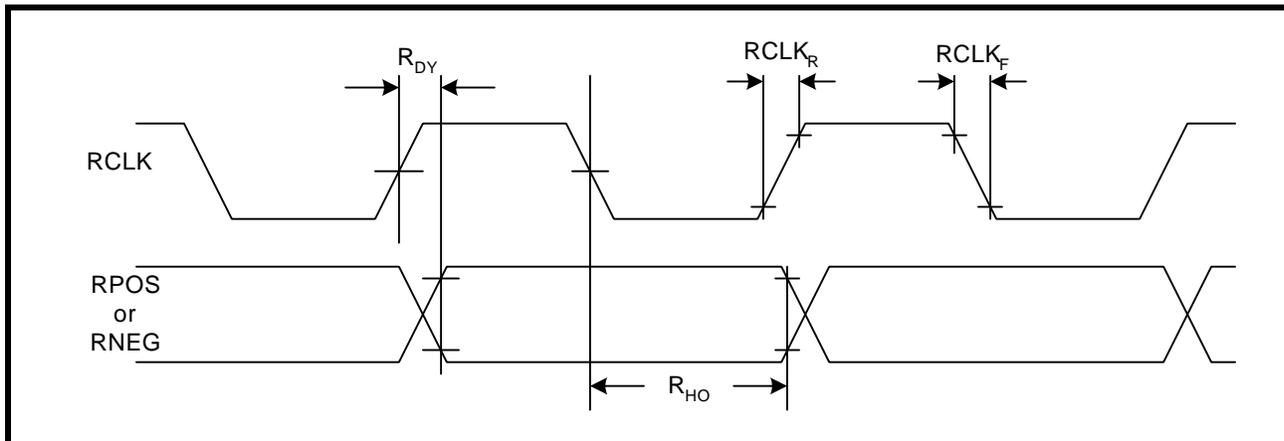
**MICROPROCESSOR INTERFACE I/O TIMING**
