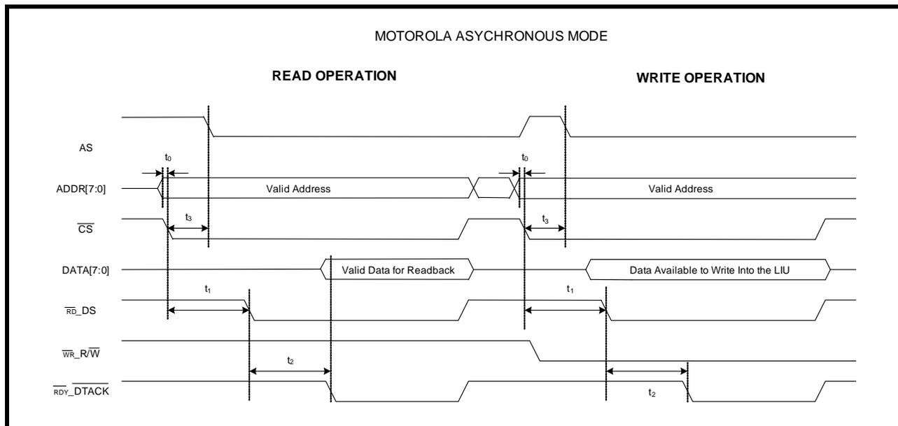
**TABLE 20: MOTOROLA 68K MICROPROCESSOR INTERFACE TIMING SPECIFICATIONS**
