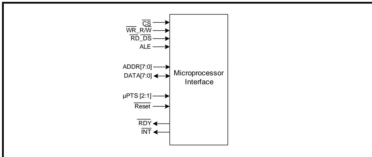
**THE MICROPROCESSOR INTERFACE BLOCK SIGNALS**
