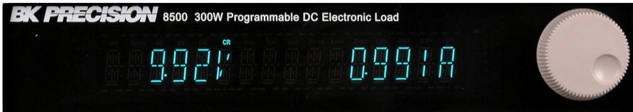
The instrument's voltage display may read a bit less than the power supply's output -- this may be due to a voltage drop in the wires connecting the power supply to the DC Load. Press the  $\Delta$  or  $\nabla$  keys to see the power that is being consumed by the load.
