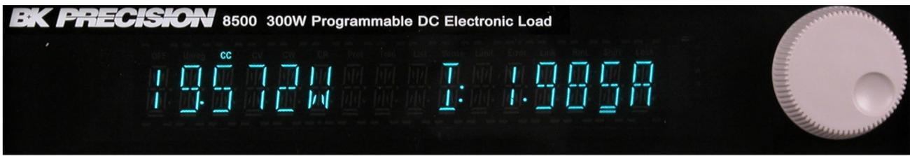
Press the **V-set** button (you may have to press it twice). Note the load is turned off. Set the power supply to 10V and the supply's current to a very low level, e.g. 0.1 A. Set the DC Load voltage level well below the supply voltage level, e.g. 1 V. Press the **On/Off** key. Verify the proper voltage level (1 V) is shown on the display. Press the  $\Delta$  or  $\nabla$  keys to see the power being dissipated.
