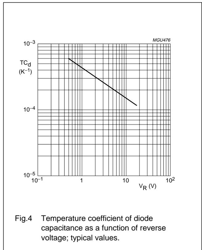
Low-voltage variable capacitance double diode
