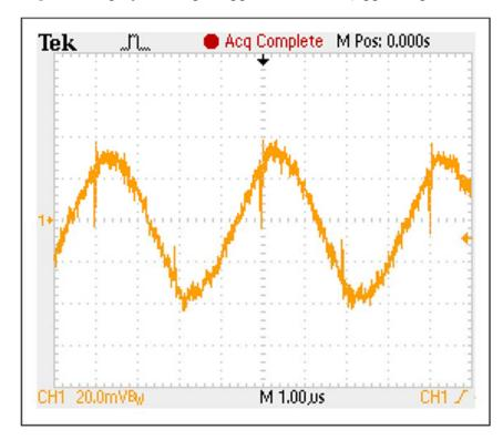
Figure 3. Output ripple at 10A load.
