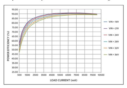
Figure 2. Power efficiency vs. load current.
