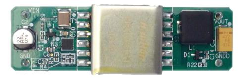
Maxim's power-supply experts have designed and built a series of isolated, industrial power-supply reference designs. Each of these power supplies efficiently converts 24V into useful voltage rails at a variety of power levels. Every power rail is isolated with a readily available transformer, providing quick, convenient transformer selection. Each design has been tested for load and line regulation, as well as efficiency and transient performance.
