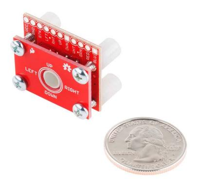
**Description:** The SparkFun BlackBerry Trackballer Breakout gives you easy access to a trackball which measures up, down, left, and right movements, clicks on the board, as well as adding a bit of flair to your project with four built-in LEDs. The trackballer breakout can be hooked into an Arduino compatible device to provide you with an intuitive direction controller.
