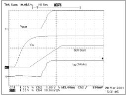
Figure 6. Start-Up Response: 5A Load
