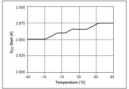
Figure 14. V<sub>cc</sub> Start Threshold vs. Temperature
