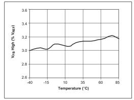
Figure 12. V<sub>FB</sub> 3% High Comparator vs. Temperature
