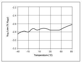
Figure 13. V<sub>FB</sub> 3% Low Comparator vs. Temperature
