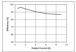
Figure 2. Efficiency vs. Output Current
