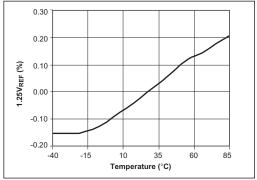
Figure 8. Error Amplifier Reference vs. Temperature
