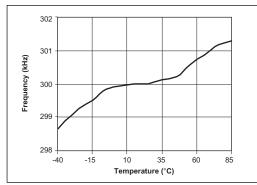
Figure 16. Oscillator Frequency vs. Temperature
