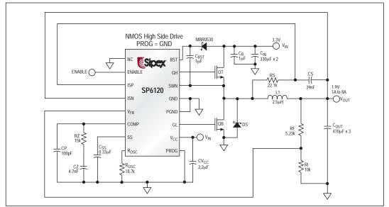
Figure 1. Schematic 3.3V to 1.9V Power Supply
