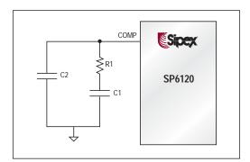
Figure 18. The RC network connected to the COMP pin provides a pole and a zero to control loop.
