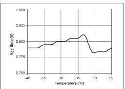
Figure 15. V<sub>cc</sub> Stop Threshold vs. Temperature
