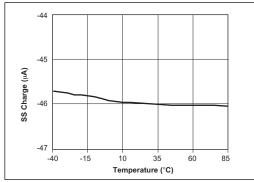
Figure 10. SS Charge Current vs. Temperature with  $V_{\rm SS} = 1.5V$
