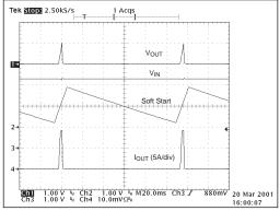
Figure 7. Overcurrent: 9A Load
