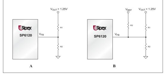
Figures 21(A), a voltage divider connected to the  $V_{_{FB}}$  pin programs the output voltageand 21(B), a simple circuit using one external voltage reference programs the output voltages to less than 1.25V.
