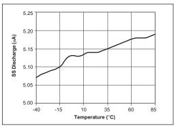
Figure 11. SS Discharge Current vs. Temperature with  $V_{\rm ss} = 1.5V$
