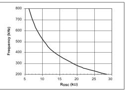
Figure 17. Oscillator Frequency vs.  $R_{osc}$  with  $V_{cc} = 5V$ and CGH = CGL = Open.
