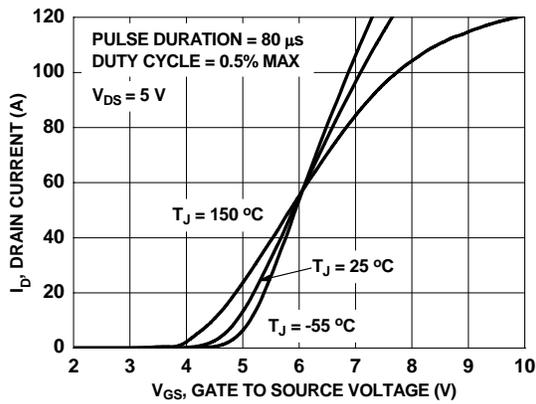
Figure 5. Transfer Characteristics
