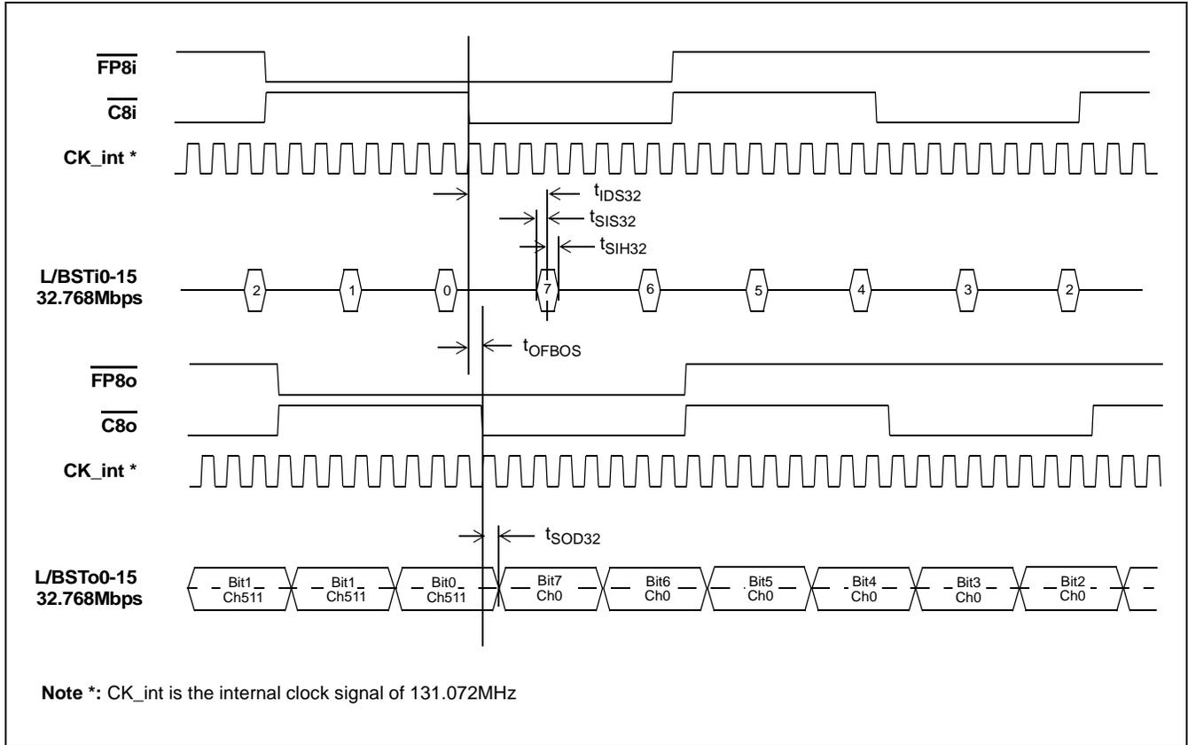
Figure 19 - ST-BUS Local/Backplane Data Timing Diagram (32Mbps)
