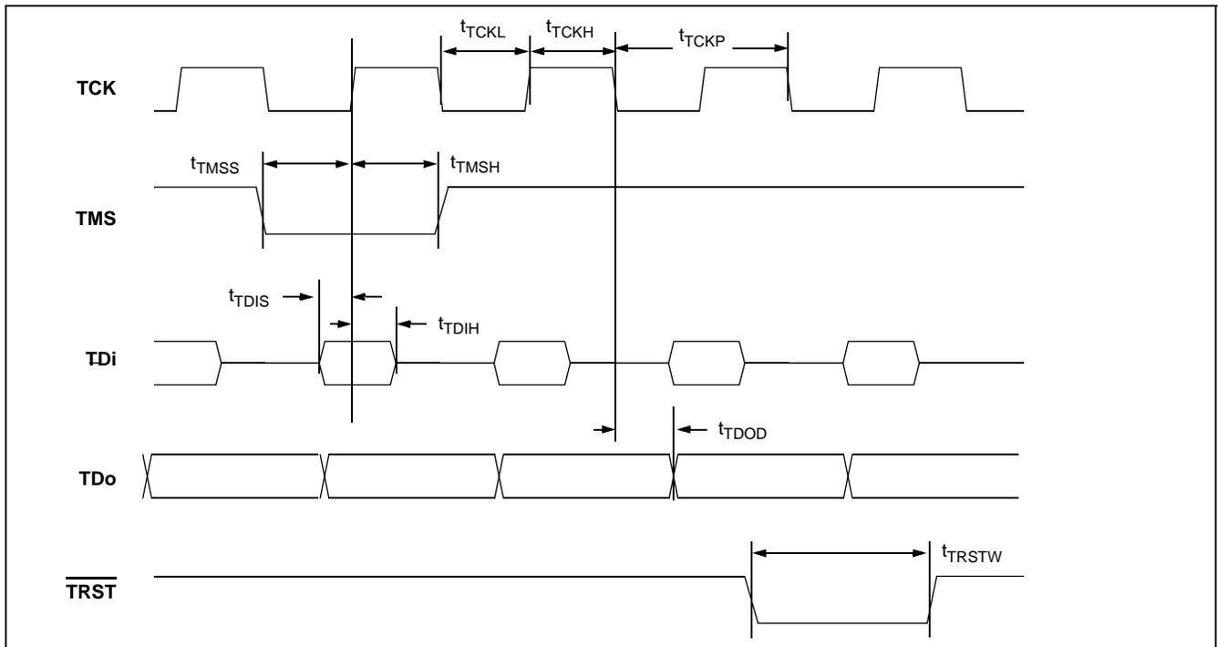
**Figure 24 - JTAG Test Port Timing Diagram**
