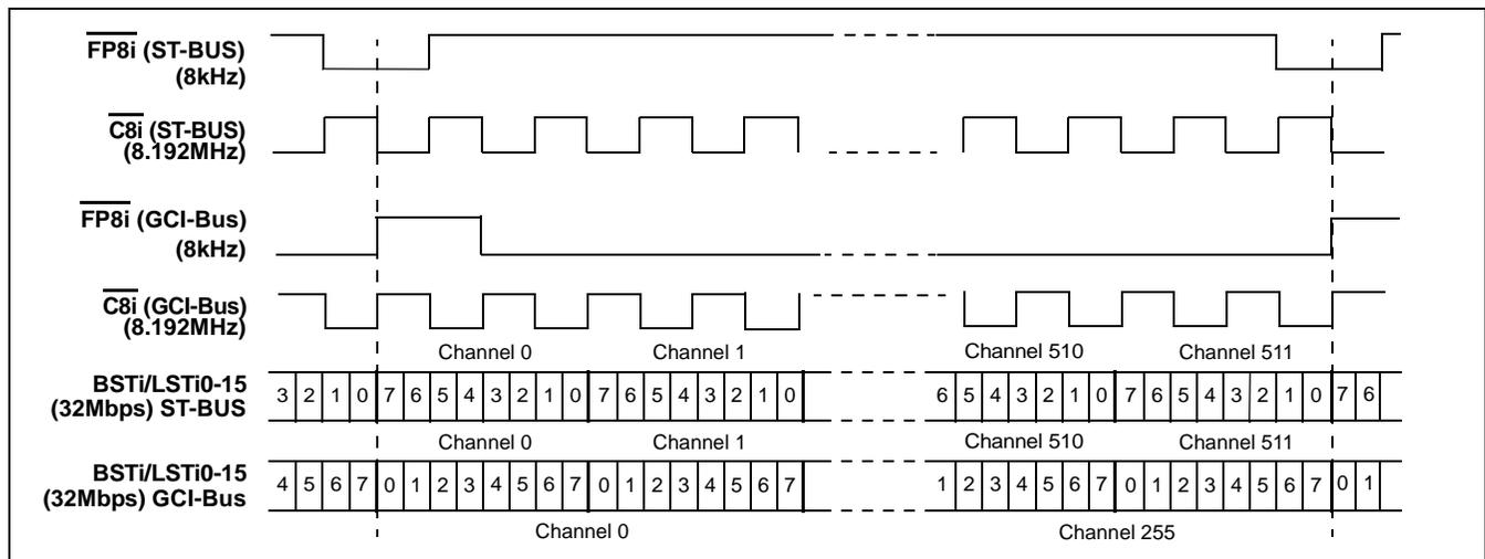
Figure 6 - ST-BUS and GCI-Bus Input Timing Diagram
