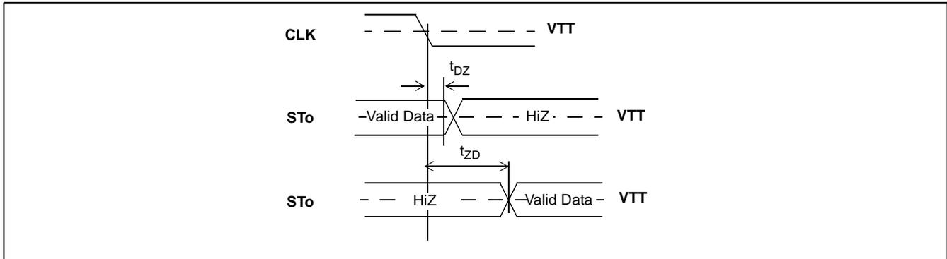
**Figure 21 - Serial Output and External Control**
