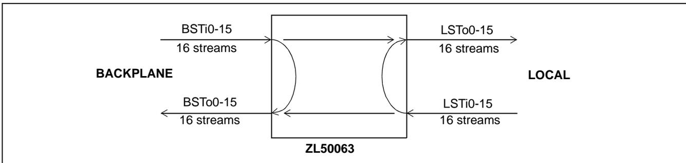
**Figure 4 - 8,192 x 8,192 Channels (32Mbps), Bi-directional Switching**
