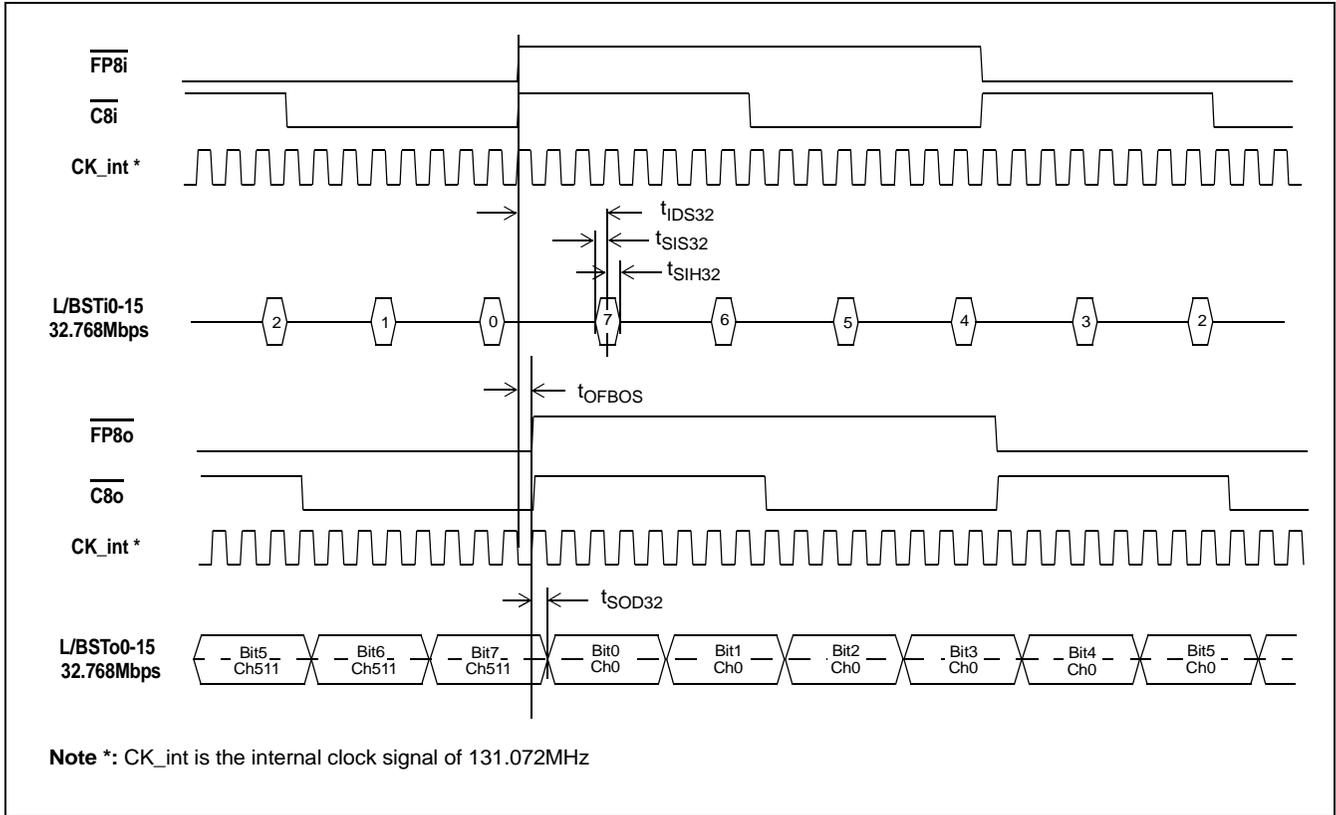
Figure 20 - GCI-Bus Local/Backplane Data Timing Diagram (32Mbps)
