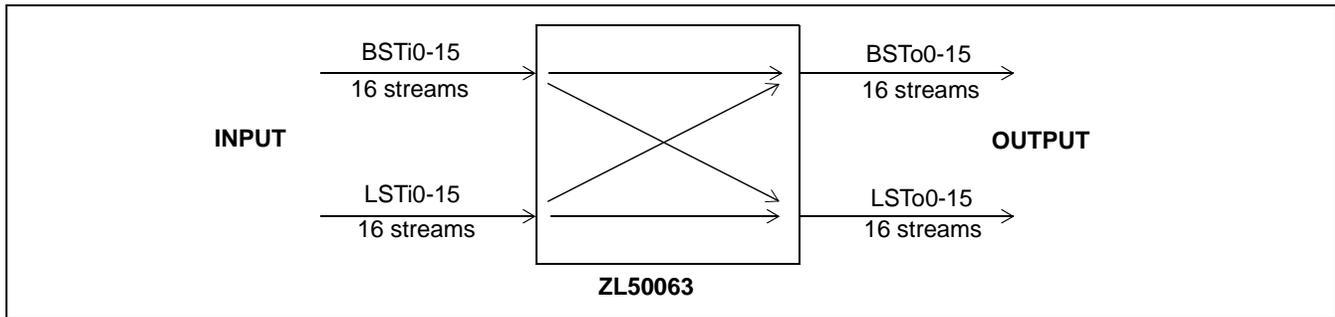
**Figure 3 - 16,384 x 16,384 Channels (32Mbps), Unidirectional Switching**
