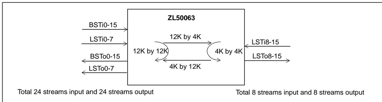
**Figure 5 - 12,288 by 4,096 Channels Blocking Bi-directional Configuration**
