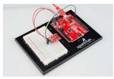
A SHT15 connected to the SDA(A4) and SCL(A5) lines on a SparkFun
