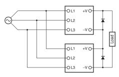
Note: 1. The diode is connected as shown in the figure. If the load is short-circuited, a reverse voltage will be generated inside the Power Supply. If this occurs the Power Supply may possibly deteriorate or be damaged. Always connect a diode as shown in the figure.
