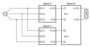
For 960 W, always connect diodes to the output sides of the two Power Supplies as shown in the following diagram.
