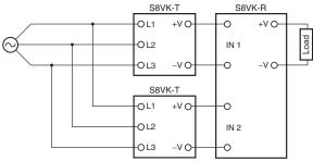
The internal parts may occasionally be deteriorated or broken. Be sure to set the OPERATION SWITCH to B when using S8VK-T 480 W, 960 W for Parallel Operation.
