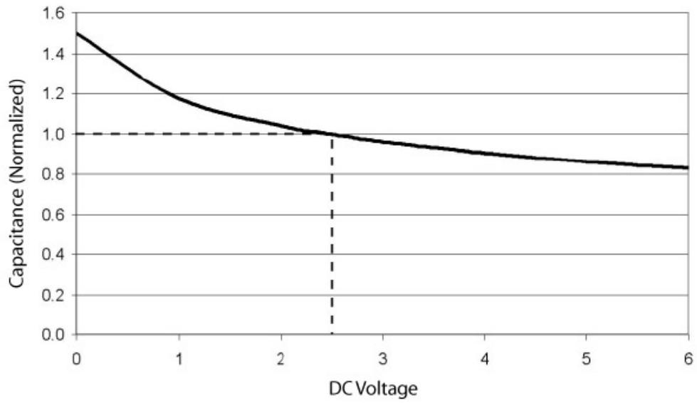
Figure 5. Filter Capacitance vs. Input Voltage
