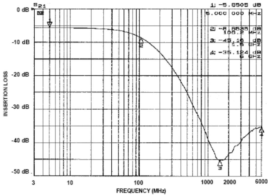
Figure 2. Insertion Loss vs. Frequency (FILTER2 Input to GND)
