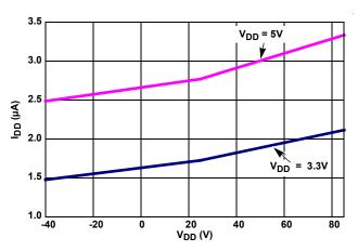
FIGURE 3. I<sub>DD1</sub> vs TEMPERATURE
