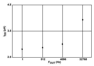
FIGURE 6. I<sub>DD1</sub> vs f<sub>OUT</sub> AT V<sub>DD</sub> = 5V
