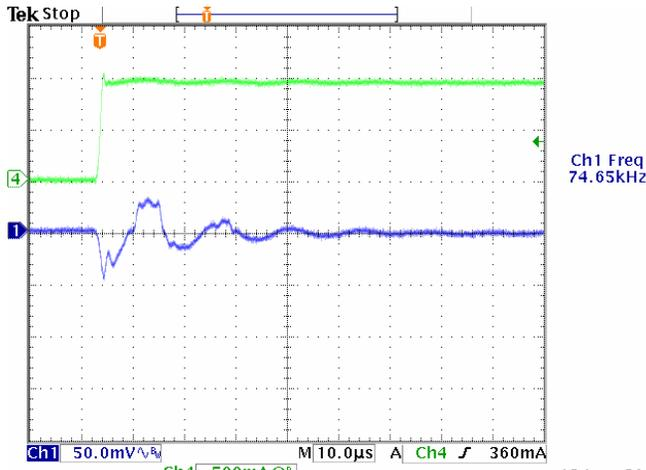
CH1:  $V_{OUT}$ , CH4:  $I_{STEP}$ ,  $C_{IN} = 10\mu F$ ,  $C_{OUT} = 10\mu F$  Ceramic,  $V_{DROOP} = 50mV$
