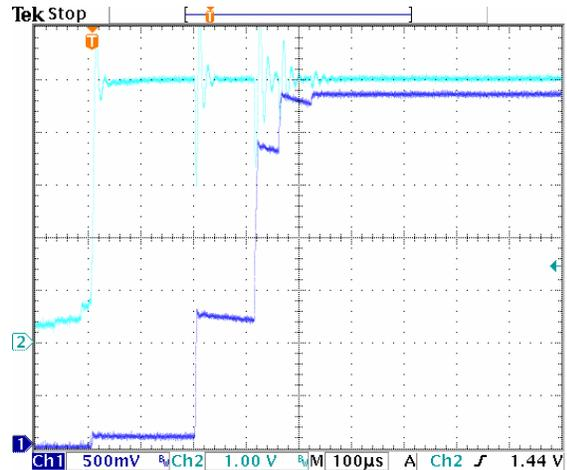
CH1:  $V_{OUT}$ , CH2:  $V_{IN}$ ,  $C_{IN} = 10\mu F$ ,  $C_{OUT} = 10\mu F$  Ceramic, Load Current, DC = 10mA
