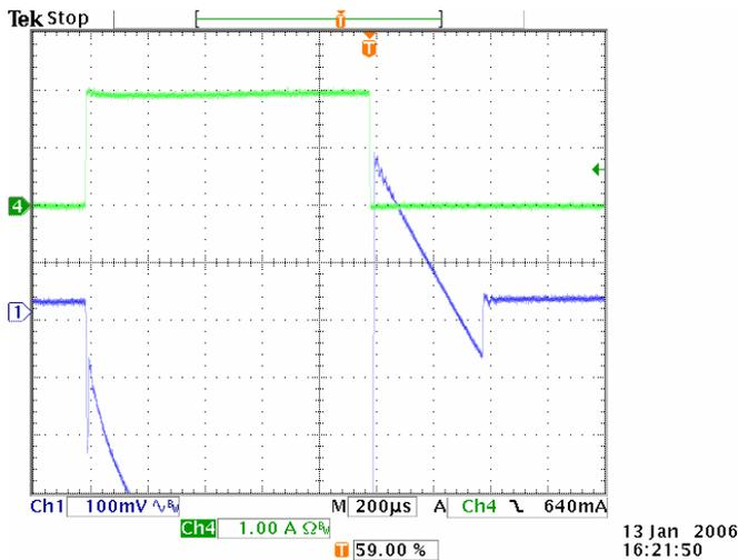
CH1:  $V_{OUT}$ , CH4:  $I_{OUT}$  1A/div,  $C_{IN} = 10\mu F$ ,  $C_{OUT} = 10\mu F$  Ceramic
