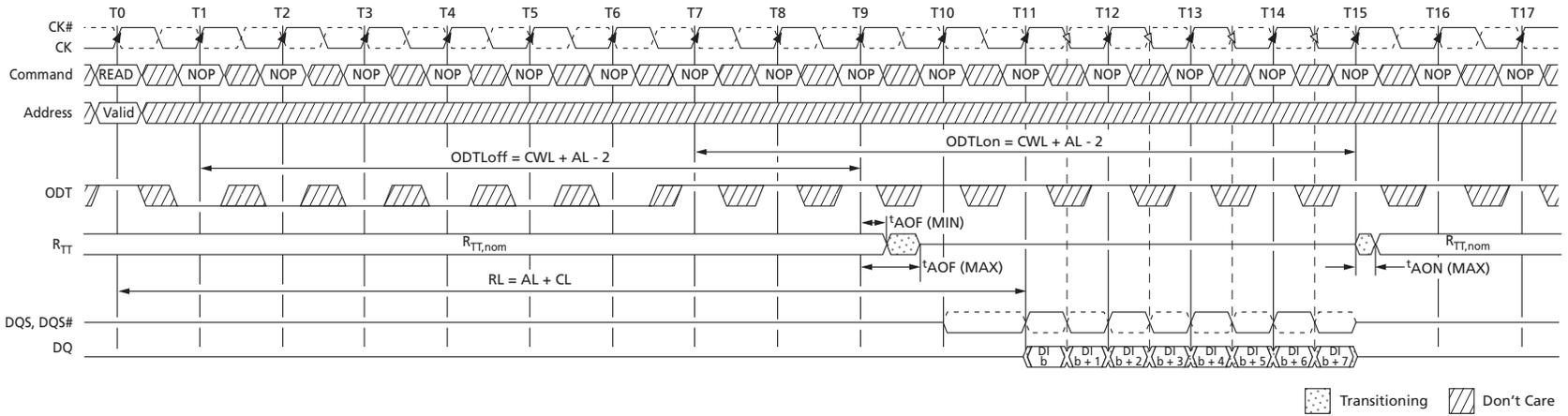
Note: 1. ODT must be disabled externally during READs by driving ODT LOW. For example, CL = 6; AL = CL - 1 = 5; RL = AL + CL = 11; CWL = 5; ODTLon = CWL + AL - 2 = 8; ODTLoff = CWL + AL - 2 = 8.  $R_{TT,nom}$  is enabled.  $R_{TT(WR)}$  is a "Don't Care."
