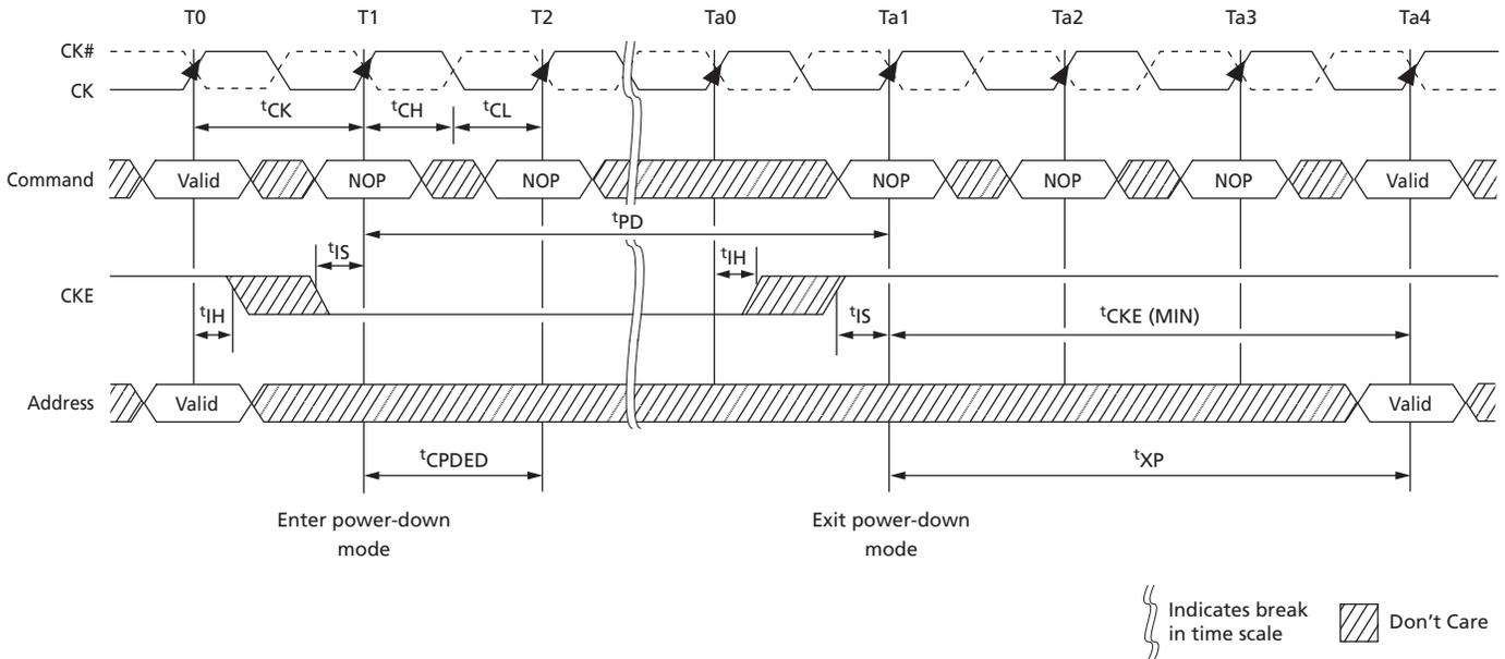
Figure 96: Precharge Power-Down (Fast-Exit Mode) Entry and Exit
