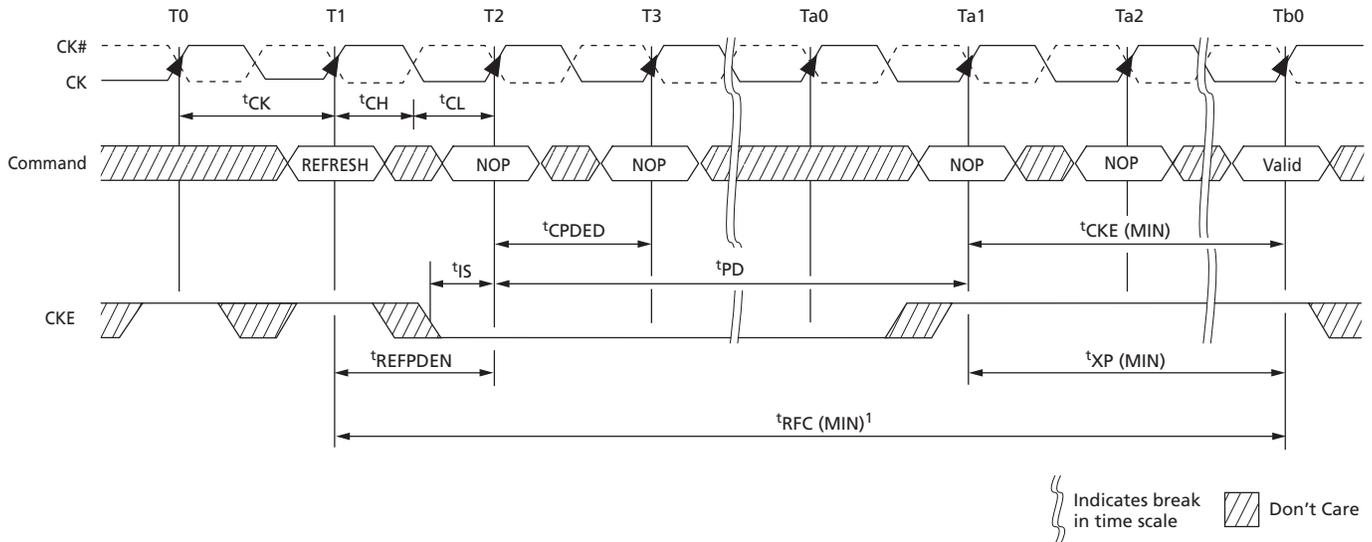
Note: 1. After CKE goes HIGH during  $t_{RFC}$ , CKE must remain HIGH until  $t_{RFC}$  is satisfied.
