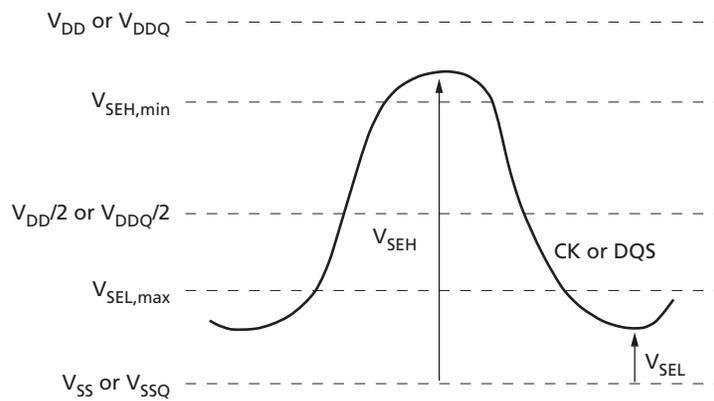
Figure 17: Definition of Differential AC-Swing and  $t_{DVAC}$
