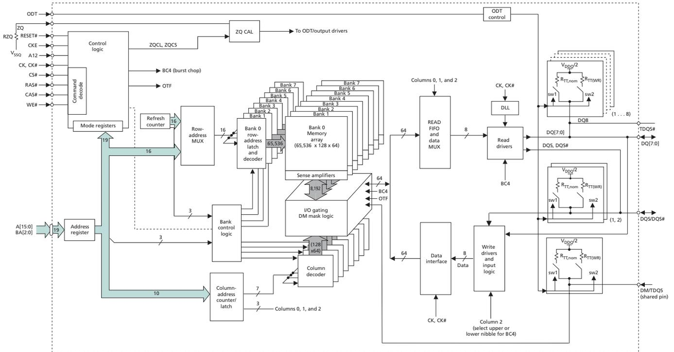
**Figure 4: 256 Meg x 16 Functional Block Diagram**
