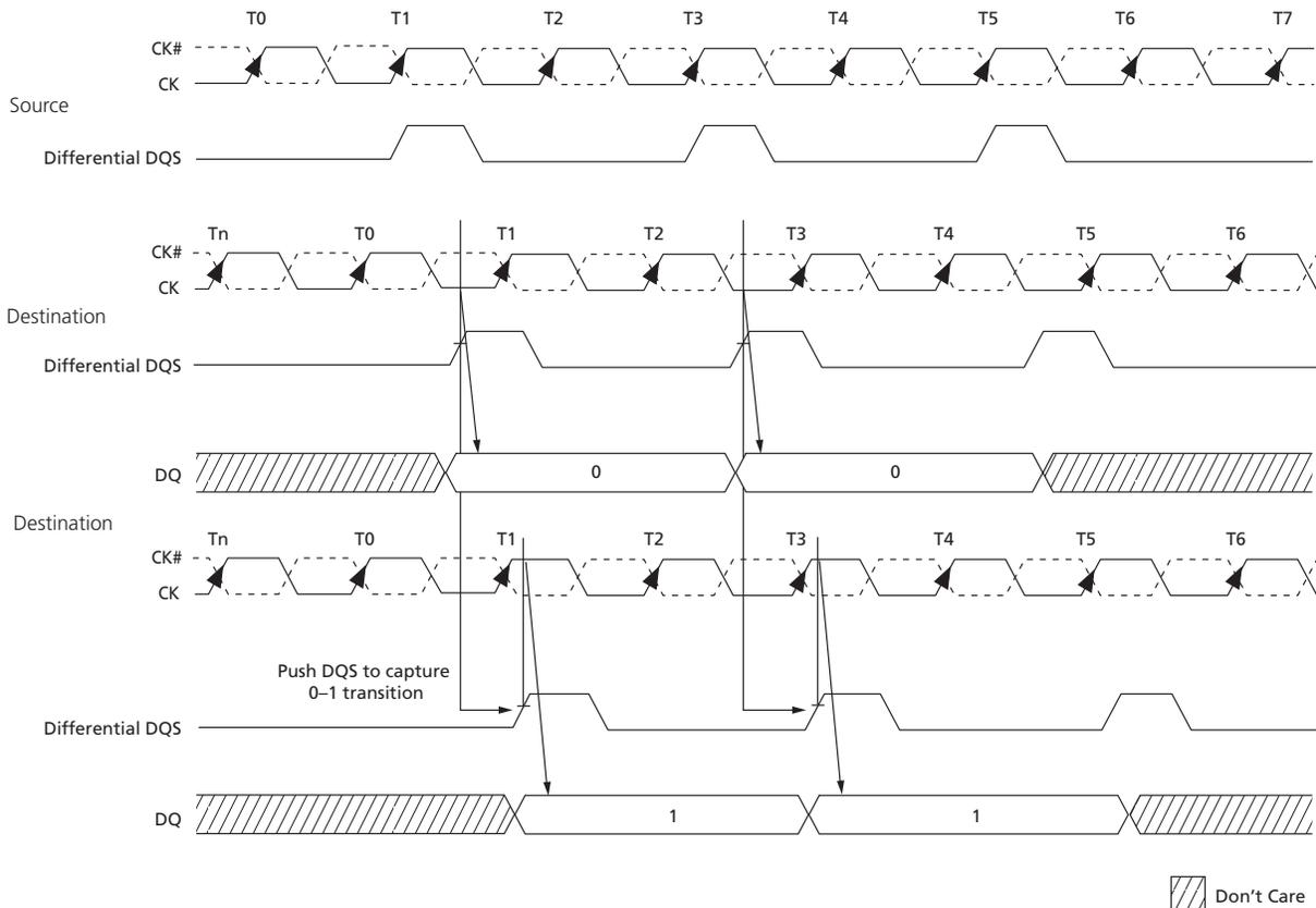
When write leveling is enabled, the rising edge of DQS samples CK, and the prime DQ outputs the sampled CK's status. The prime DQ for a x8 configuration is DQ0 with all
