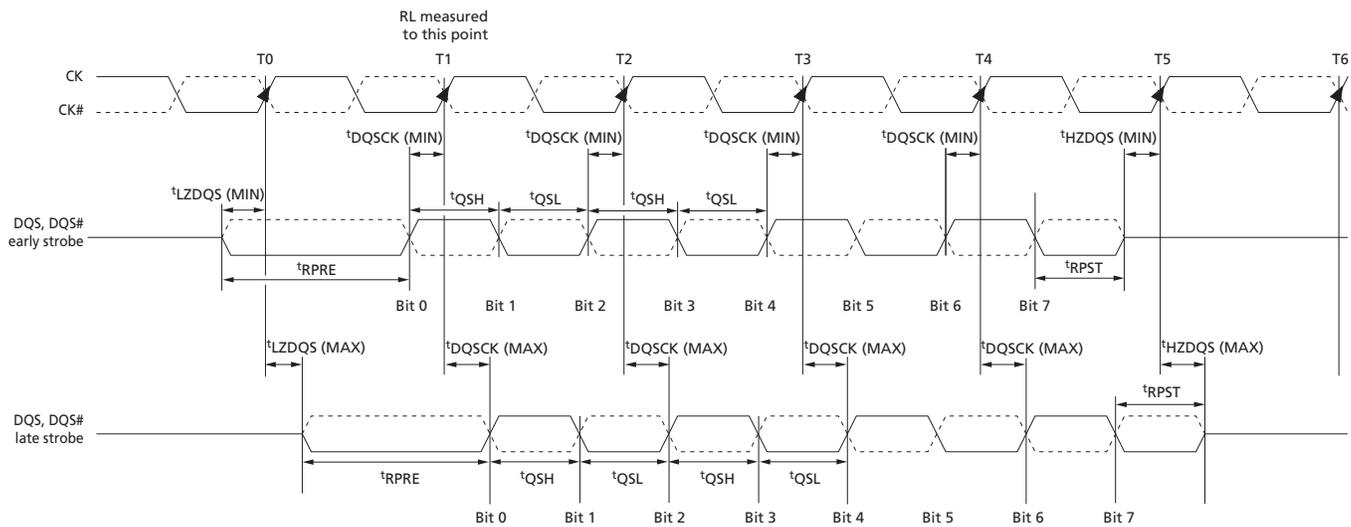
**Figure 78: Method for Calculating  $t_{HZ}$  and  $t_{LZ}$**
