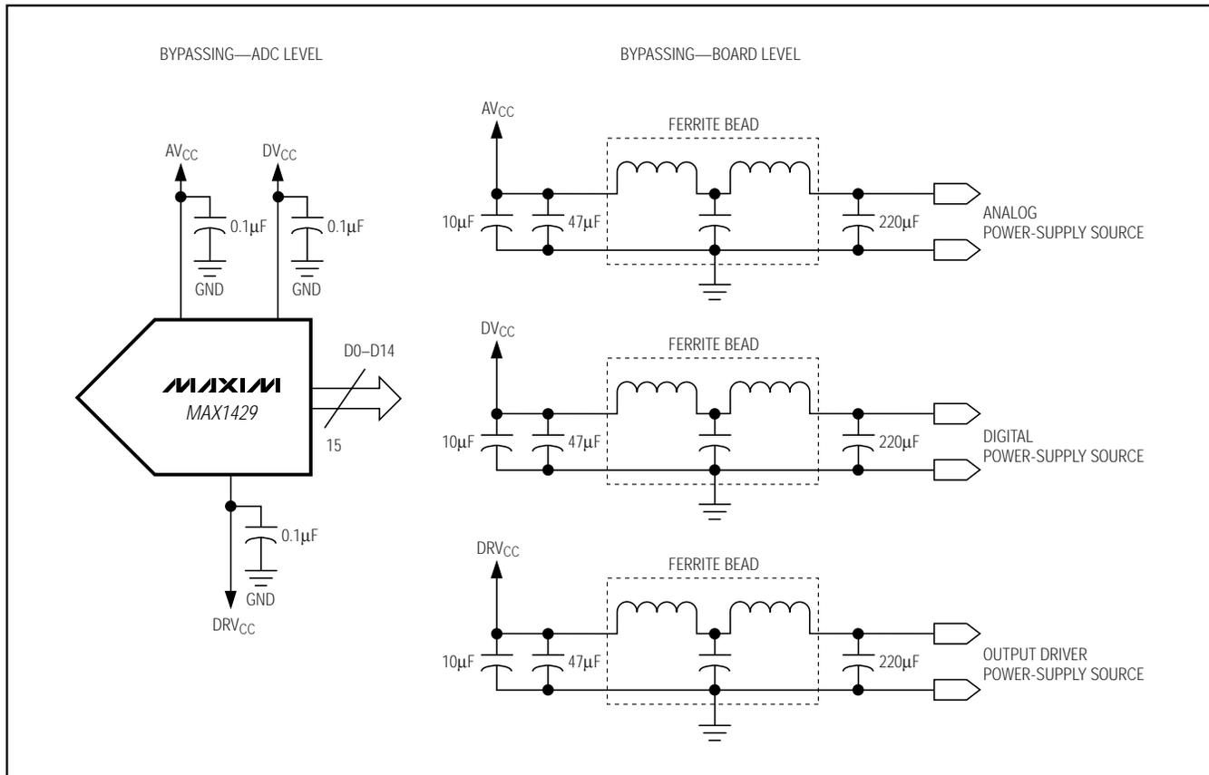
Figure 9. Grounding, Bypassing, and Decoupling Recommendations for MAX1429
