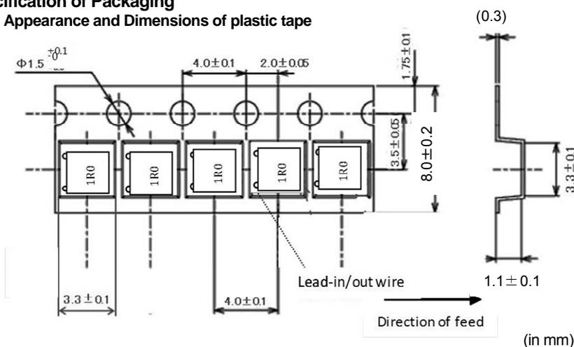
Dimension of the Cavity is measured at the bottom side.
