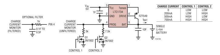
Figure 2. Logic Control Programming of Output Current to OmA, 200mA, 500mA or 700mA
