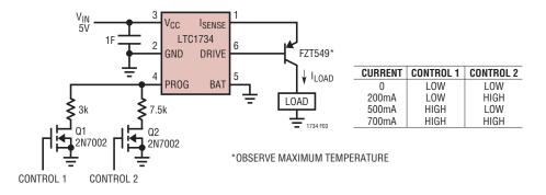
Figure 3. Programmable Current Source with Output Current of OmA, 200mA, 500mA or 700mA
