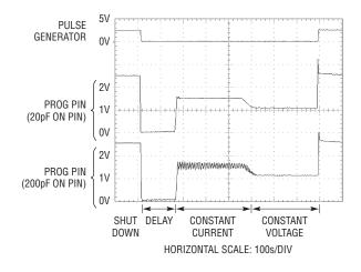
Figure 5. Stability Waveforms
