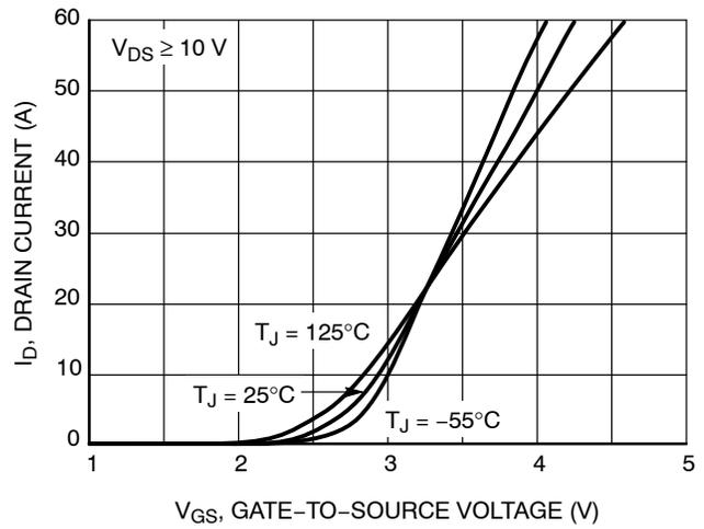
Figure 2. Transfer Characteristics
