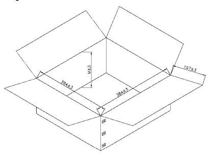
M = H(Capacitor height) + Terminal height + 10mm min.
