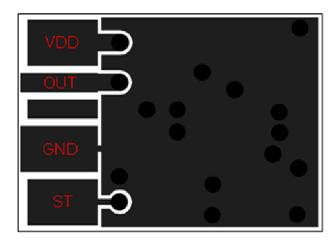
Figure 3: SiT6303EB layout (Bottom side)
