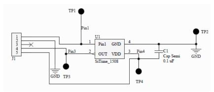
Figure 1: SiT6303EB r. 1.0 schematic
