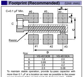
source terminal of the crystal products (between VCC - GND).
