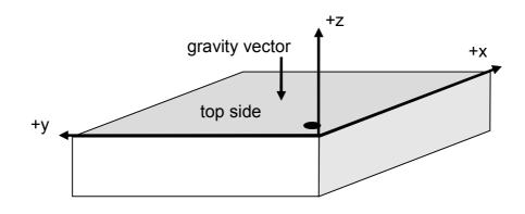
The following table lists all corresponding output signals on Ax, Ay, and Az while the sensor is at rest or at uniform motion in a gravity field under assumption of a top down gravity vector as shown above.
