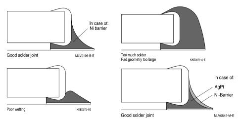
Good and poor solder joints caused by amount of solder in reflow soldering.
