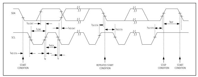
Figure 2. Serial-Interface Timing Details
