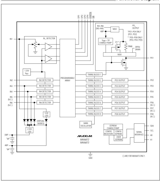
Program each output to assert on any voltage-detector input, general-purpose logic input, watchdog timer, manual reset, or other output stages. Programmable timing-delay blocks configure each output to wait between 25µs and 1600ms before deasserting. A fault register logs the conditions that caused each output to assert (undervoltage, overvoltage, manual reset, etc.).
