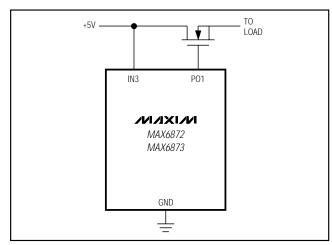
Figure 9. Driving High-Side n-Channel MOSFET Switches
