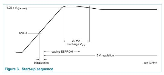
The TEA19051BT operates on supply voltages up to 21 V. The voltage on the VCC pin is used to detect an OVP and UVP. The OVP and UVP level are set as a percentage of the requested output voltage level.
