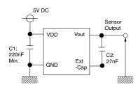
The frequency characteristics value can be changed depending on the C2 capacitance value.
