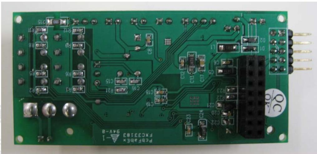
Figure 2 – Bottom view of ISD-DEMO15D00 Rev-A board
