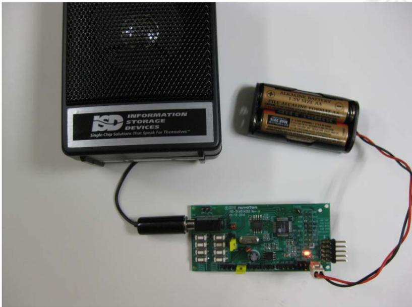
Figure 8 – ISD15D00 demo board standalone evaluation.
