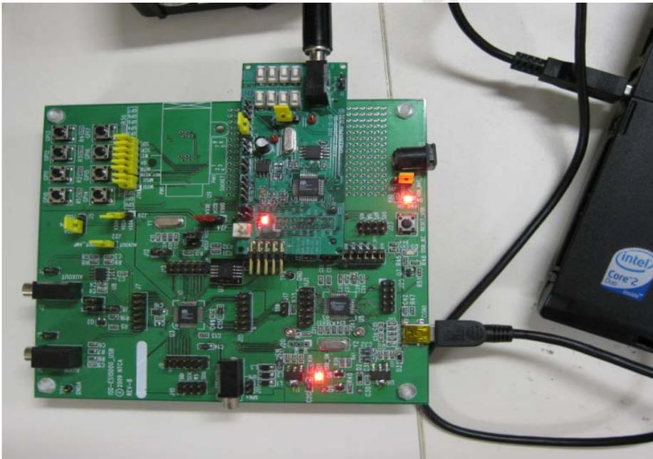
Figure 6 – ISD15D00 is connected onto ISD-ES15D00\_USB mother board
