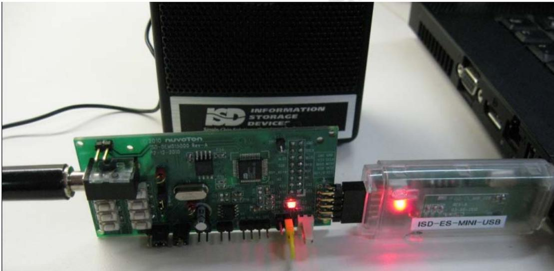
Figure 4 – A complete evaluation environment for ISD15D00 device
