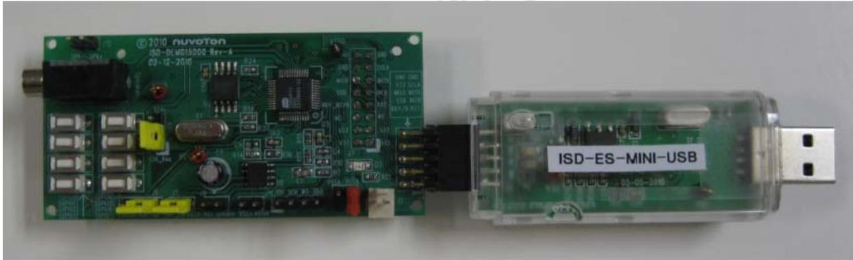
Figure 3 – ISD\_DEMO15D00 connected with ISD-ES\_MINI\_USB (dongle) board
