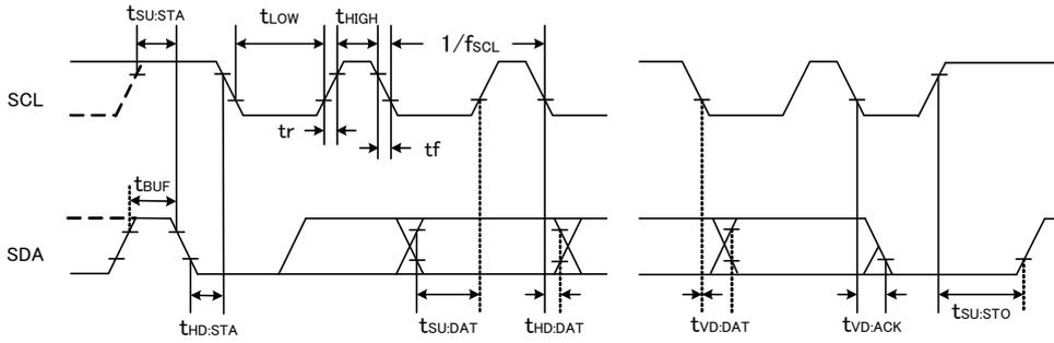
Fig.3 Definition of logic signal timing
