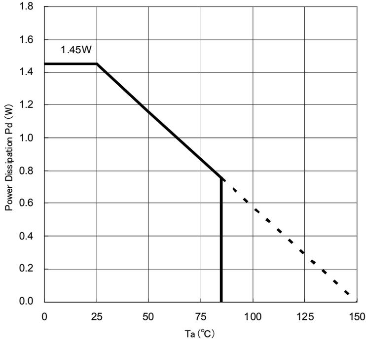
Fig. 9 Power dissipation
