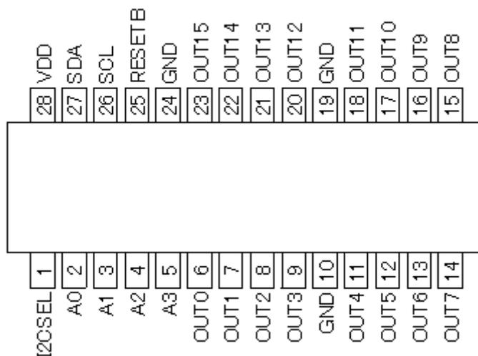
Fig.2 Pin arrangement
