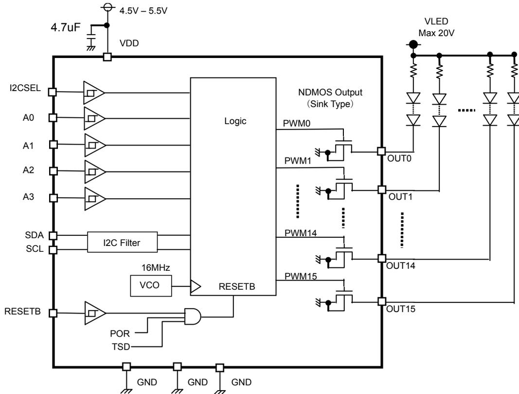
Fig.1 Block Diagram / Application Circuit example
