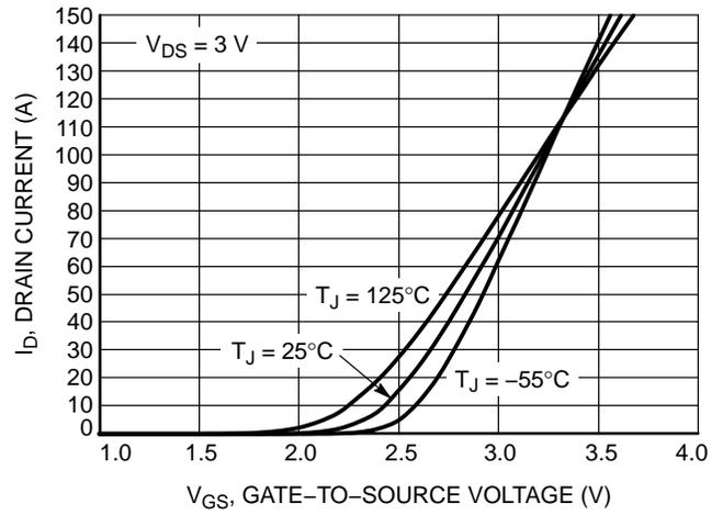
Figure 2. Transfer Characteristics
