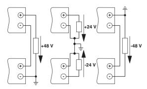
Figure 29 Schematic diagrams in series operation
