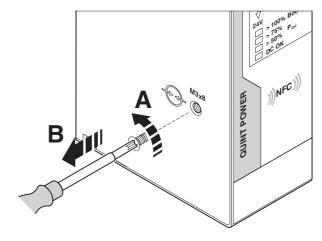
Figure 2 Disconnect gas-filled surge arrester
