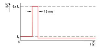
Figure 21 SFB pulse trips circuit breakers
