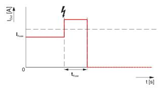
Figure 18 FUSE MODE output characteristic curve
