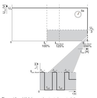
Figure 16 U/I Advanced output characteristic curve
