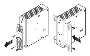
Figure 12 Mounting the UWA 130 universal wall adapter
