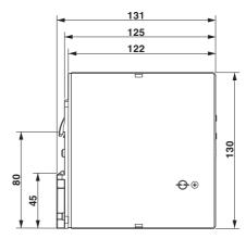
Figure 5 Device dimensions (in mm)
