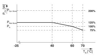
Figure 33 Derating in the static boost
