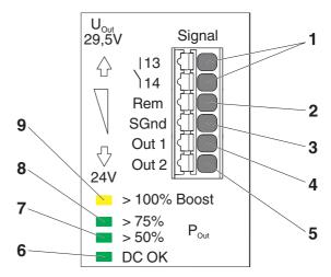
Figure 23 Position of the signaling element
