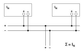
Figure 30 Schematic diagram in parallel operation
