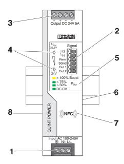
Figure 3 Operating and indication elements
