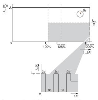
Figure 17 Smart HICCUP output characteristic curve
