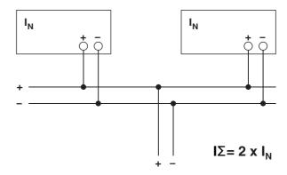
Figure 32 Schematic diagram of increased performance
