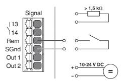
Figure 25 External wiring versions, disable SLEEP MODE
