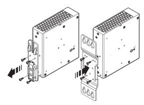
Figure 11 Mounting the UWA 182/52 universal wall adapter
