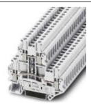
Double-level terminal block, connection method: Screw connection, cross section: 0.14 mm² - 4 mm², AWG: 26 - 12, width: 5.2 mm, color: white, mounting type: NS 35/7,5, NS 35/15
