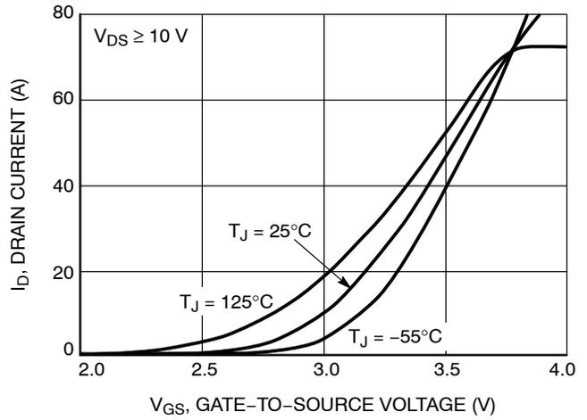
Figure 2. Transfer Characteristics
