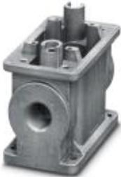
HEAVYCON ADVANCE B6 coupling housing, for M6 screw locking, salt-water-resistant aluminum, with 1 x M20 thread, straight cable outlet, without surface coating
